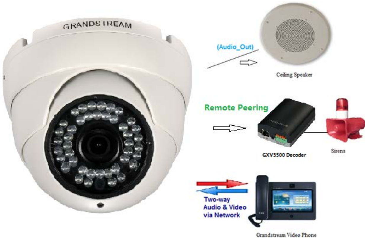
Figure 6: Application Peripheral Connection for GXV3610_HD/FHD v2
